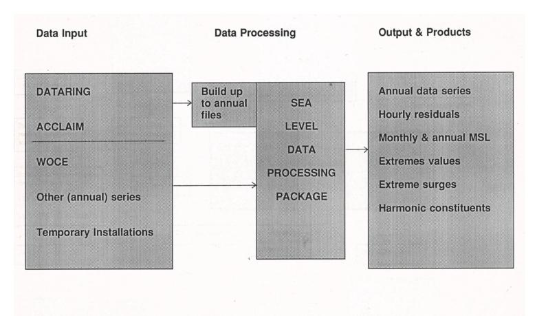
Figure 4: Overview of Sea Level Processing Package
