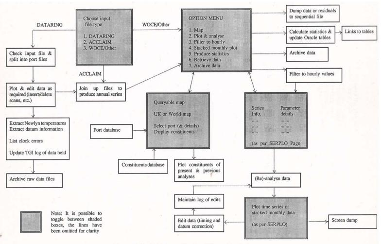
Figure 5: Detailed view of Sea Level Processing Package
